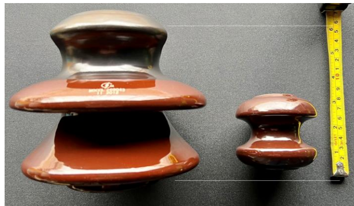
Example of an 11kV High Voltage insulator (left) with a Low Voltage insulator (right) showing the size comparison between HV & LV insulators.
