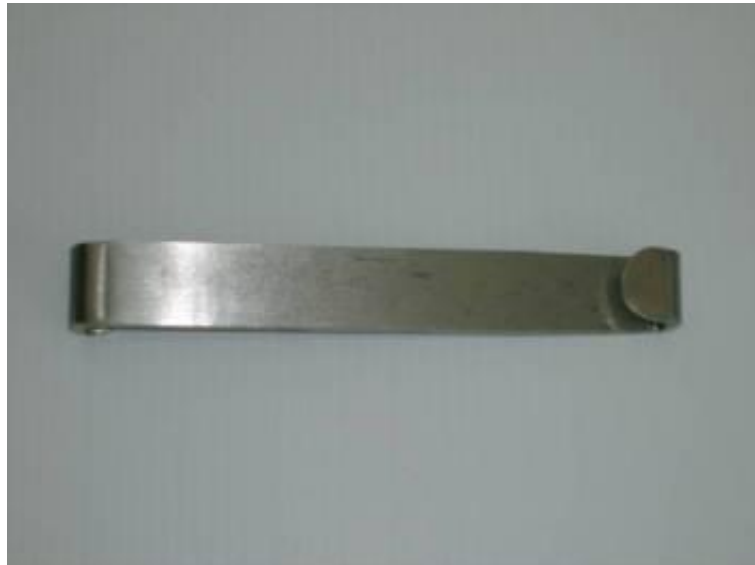
Figure 10: Above: The Keyhole Insertion Safety Shim (KISS tool), Item Code 056488
