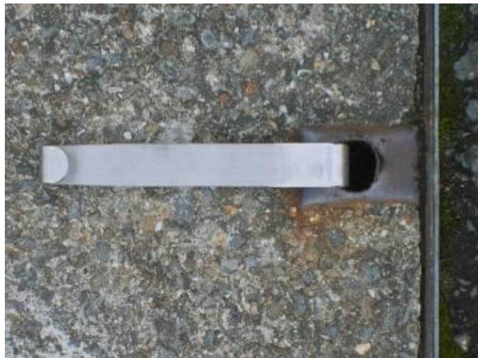
Figure 14: Inserting the KISS tool into a Worn Keyhole.
