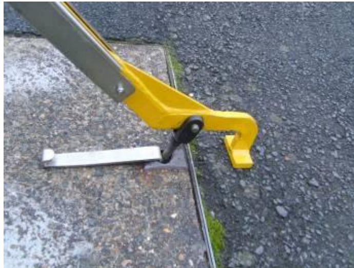
Figure 15: Key Joint Box No.5 and KISS tool.
