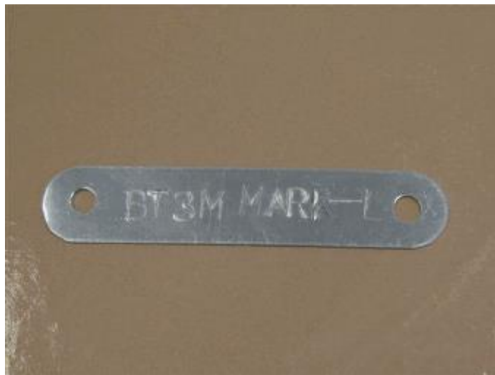
Figure 5- Aluminium strip close up, showing owner (BT) 3m mark and gauge 'L'
