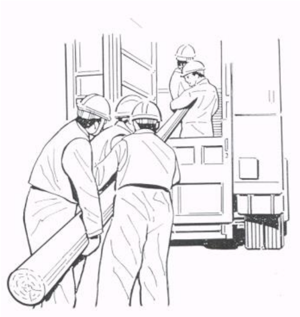
Figure 13: Loading Pole onto Vehicle (2)
